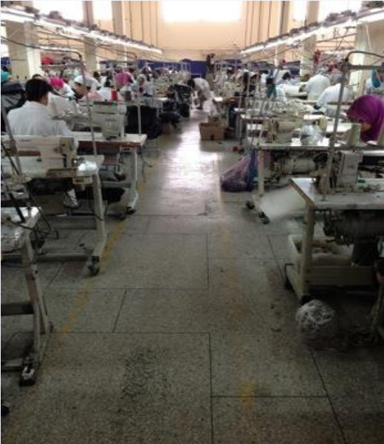
Evacuation routes in many sections should repainted
