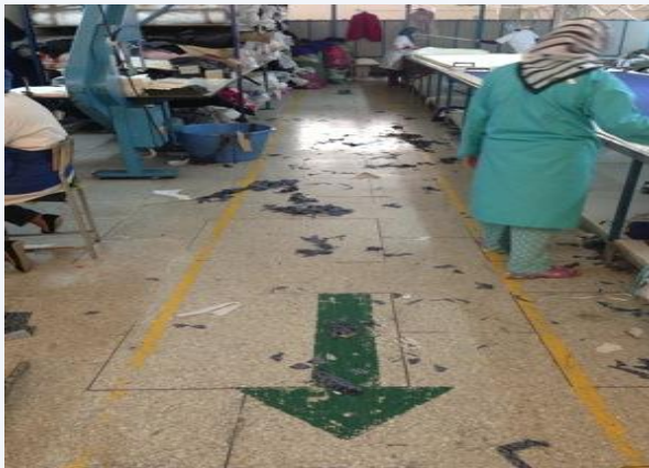
Evacuation routes painted on the floor with arrows leading to fire emergency exits
