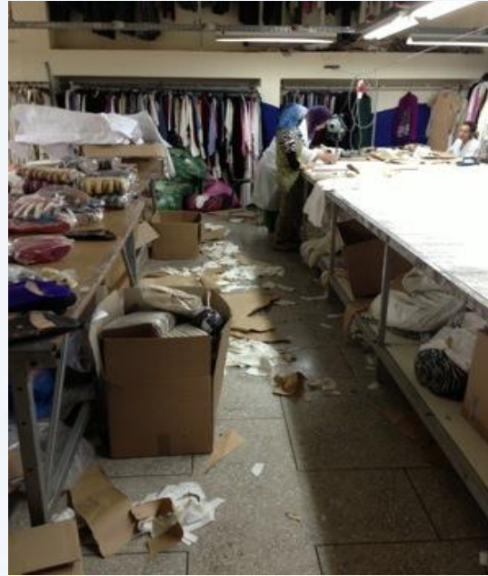
Poor housekeeping + No evacuation route painted on the floor + Escape route obstructed
